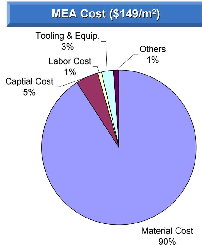
**In 2005, the MEA cost was higher due to higher material costs for the membrane (2 mil), electrodes (Pt loading = 0.75 mg/cm<sup>2</sup>) and GDL (woven carbon fiber = \$30/kg).**
