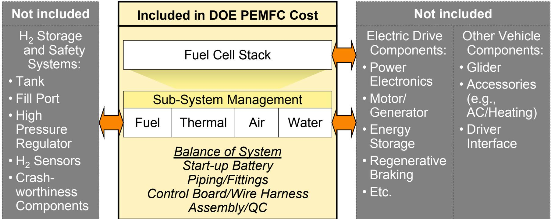
**Quality Control (QC) includes leak and voltage tests, but does not include stack conditioning.**
